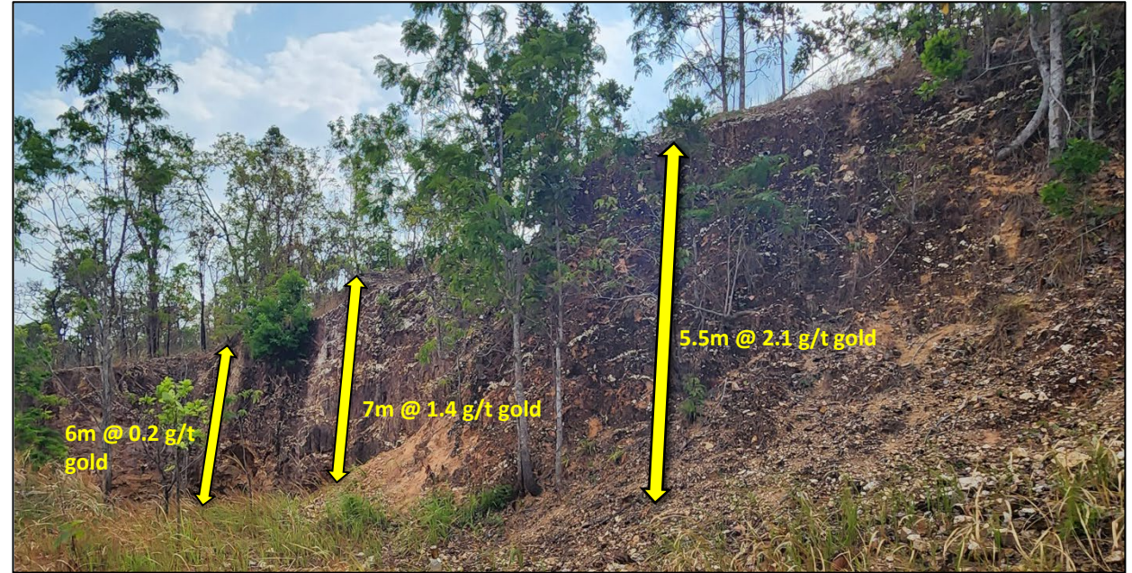
Unity channel sampling of stockwork mineralisation at Camp Prospect
