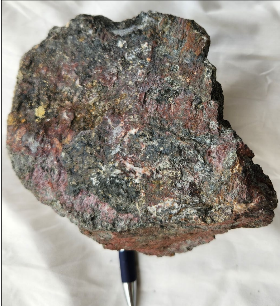
Diorite with quartz breccia veins and disseminated chalcopyrite grading 44g/t gold, 119g/t silver & 1.1% copper from Okvau Mine Corridor within the Ngot licence
