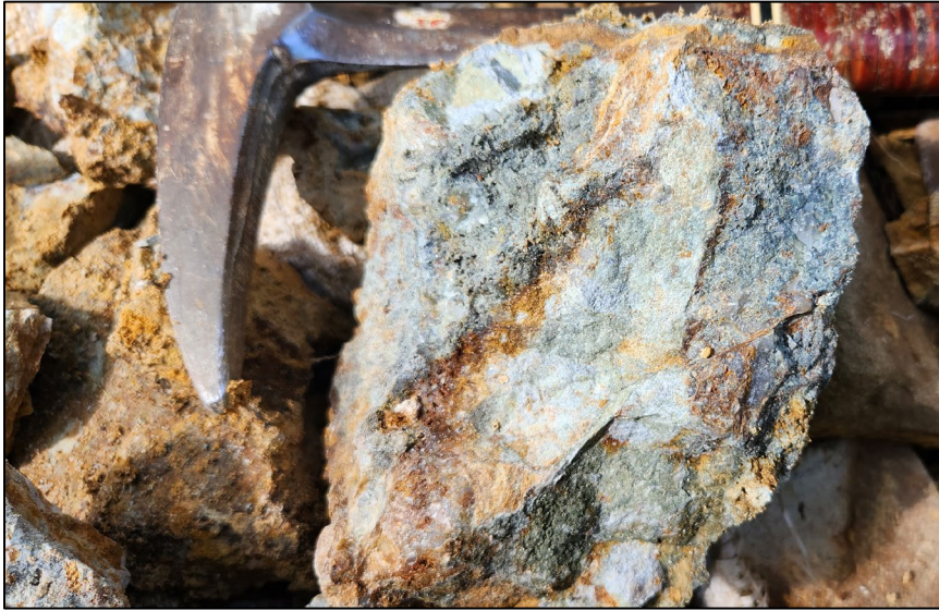
Sheeted quartz-arsenopyrite mineralisation (this Unity rock chip sample assayed 26.9g/t gold & 17.8% arsenic)
