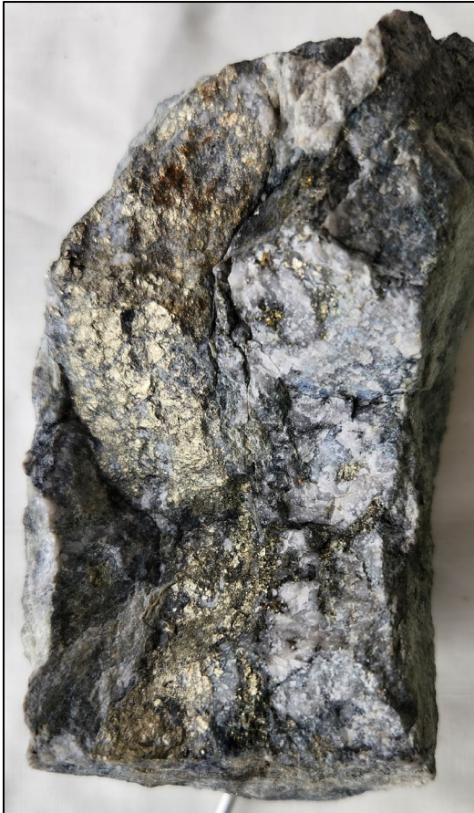
Mineralisation located 200m north of Ngot boundary assaying 6.2g/t gold, 202g/t silver & 1.3% copper
