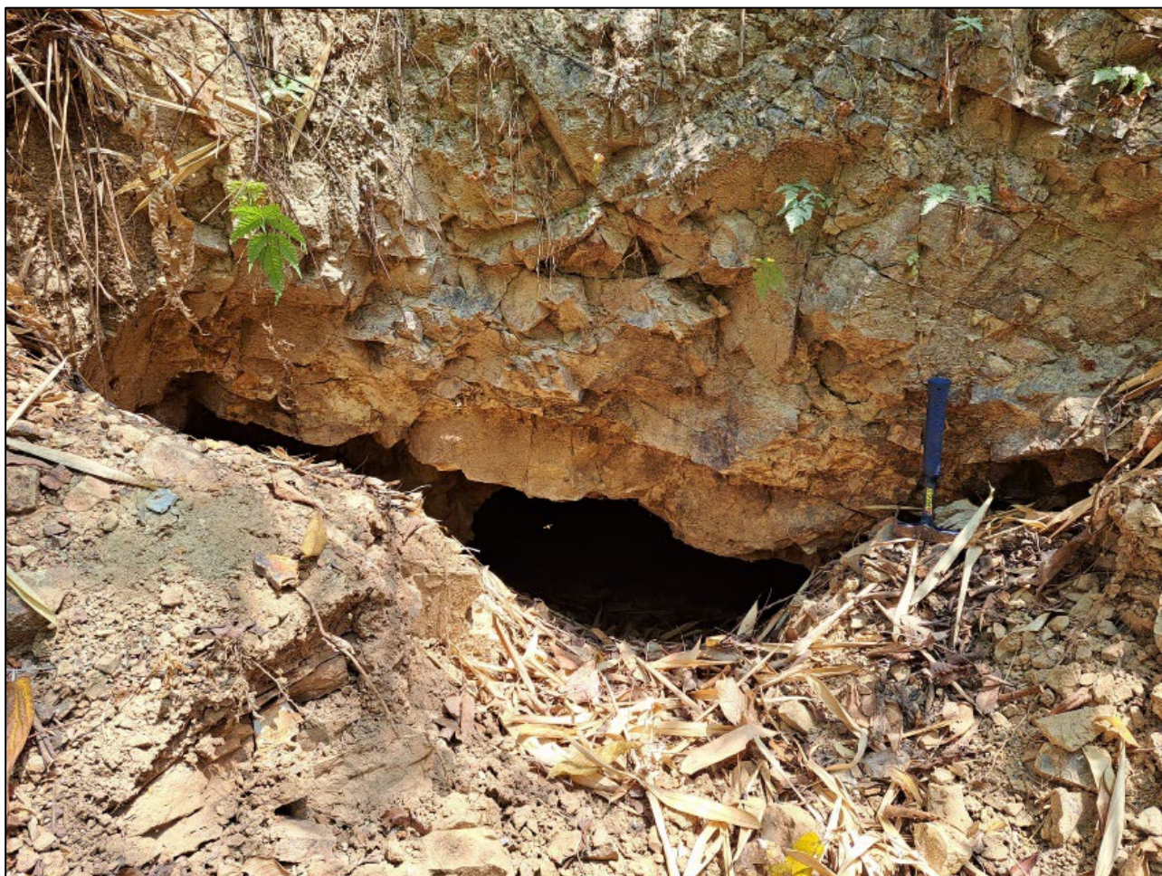
Photograph 1. Rohav Prospect – Vietnamese artisanal mine adit on a flat-lying stacked gold vein.
