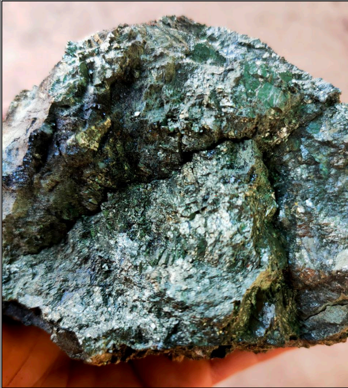
Photograph 2. Rohav Prospect - vein material (massive pyrite-arsenopyrite-sphalerite) collected from a mullock dump located outside one of the Vietnamese adits, which assayed 24.7g/t gold, 206g/t silver, 0.9% lead & 4.4% zinc.
