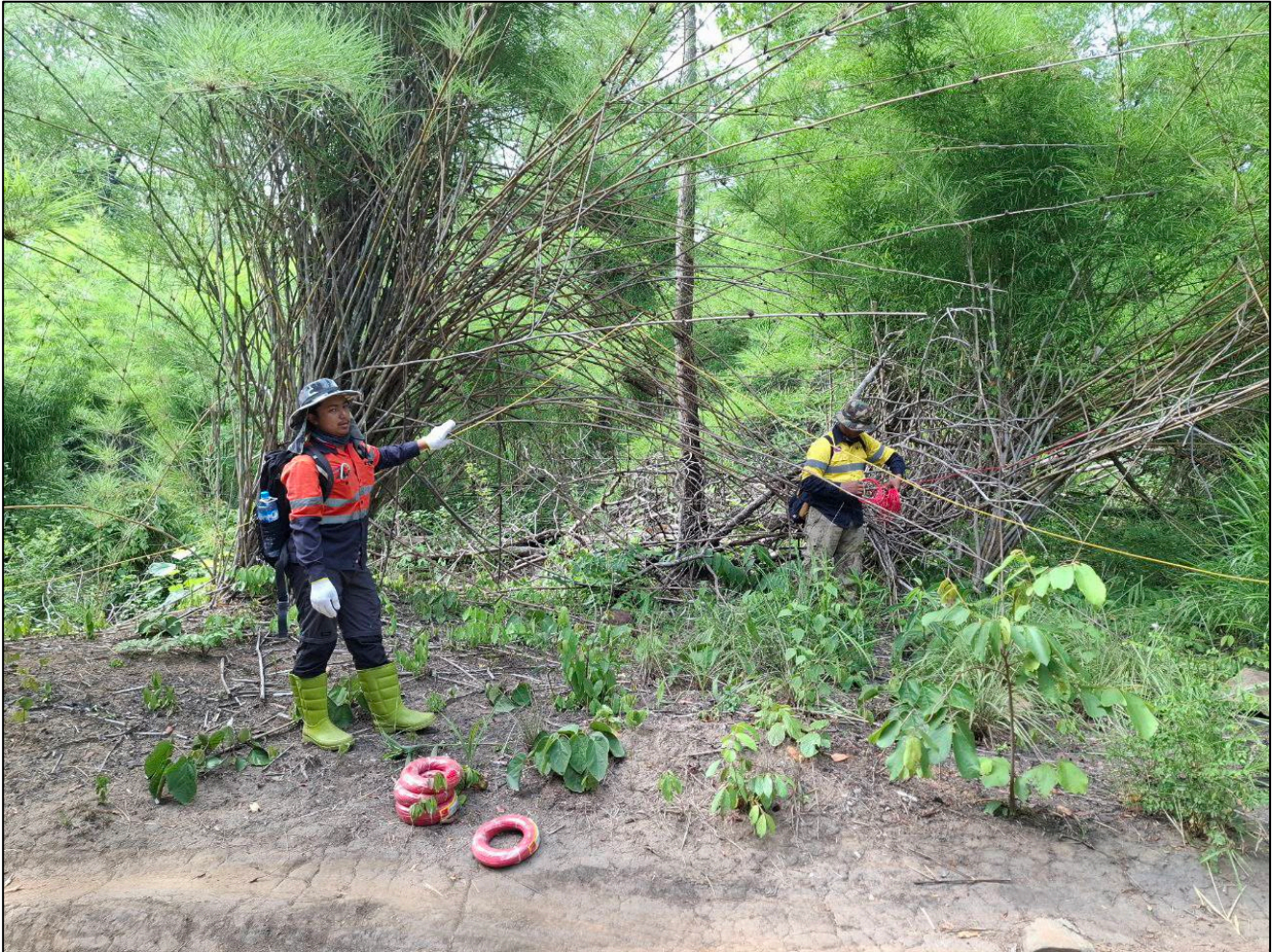
Photograph 1. Rohav Prospect – setting up the Tx wire on Line 1391000N for the dipole-dipole IP survey.
