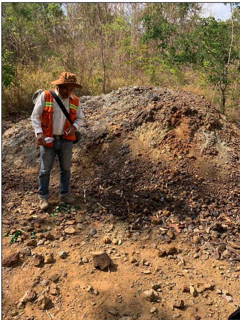
Photo 7. Arsenopyrite-rich mullock adjacent to an old mine working at the Small Creek prospect. A rock chip sample from this material returned 10.7g/t gold.
