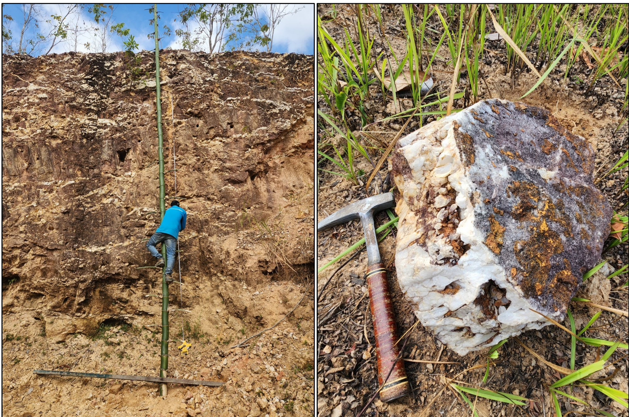
Photos 3 & 4. Channel rock chip sampling of the intense stockwork mineralisation which is exposed in pit walls associated with the Chinese mine workings south of the historical prospecting plant at the Camp prospect (LHS); & one of the thicker quartz veins from the granodiorite-hosted stockwork mineralisation with large quartz crystals terminating in an open void in the centre of the vein (RHS).
